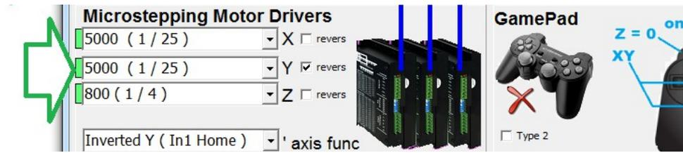
The program is marked in green for suggested values for previously specified axis ratios for fast and precise positioning. Red mean not recommended microstepping for your gears.
