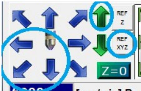
Lift the Z-axis upwards, the X-axis upwards to the Left and the Y-axis downwards (to yourself) and click REF XYZ.
