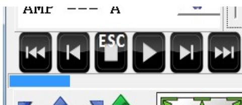
Automatic operation buttons - Scroll the program to any path (also possible by moving the blue progress indicator), stop and start the program. Holding down the **SHIFT** key, the program will be started without switching on the torch (**cutting simulation – machine will move only**).
