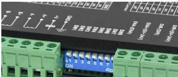
**WARNING !!!! Configuration of the controller steps division (usually set by means of microswitches / see the controller's manual) must be consistent with the settings in the program!!!!**
