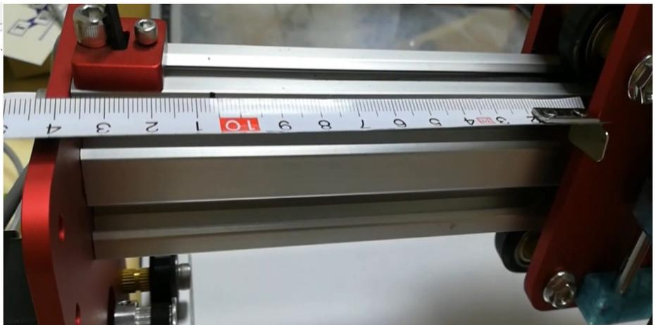
**Tip: According to MyPlasm CNC users, the best results (high dynamics, speed and precision) are obtained with identical X,Y axis ratios within the range of 30-80mm feed rate per motor revolution and 8-20mm per motor revolution for the Z axis.**
