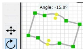
The rotation tool while holding the **CTRL** key forces a 5 degree rotation
