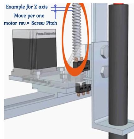
For the **Z axis**, this is usually the pitch of the drive screw thread, taking into account possible gear ratios.
